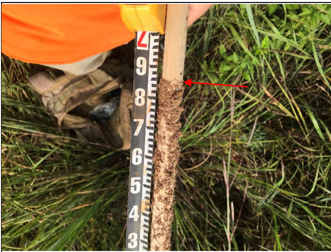
Crest Gauge Reach UT4-R2: Overbank event of 1.86' (photo from 8/12/20)
