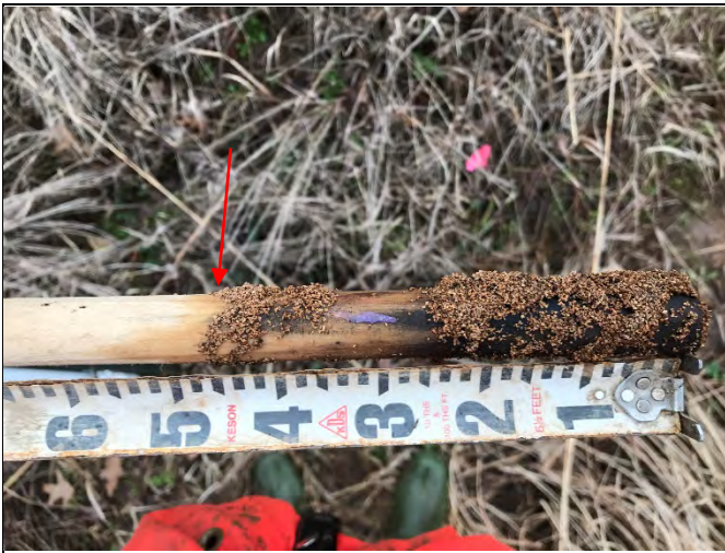
Crest Gauge Reach UT4-R2: Overbank event of .47' (photo from 2/24/20)
