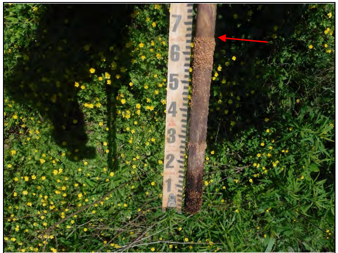
Crest Gauge Reach HC-R1: Overbank event of .65' (photo from 4/16/20)
