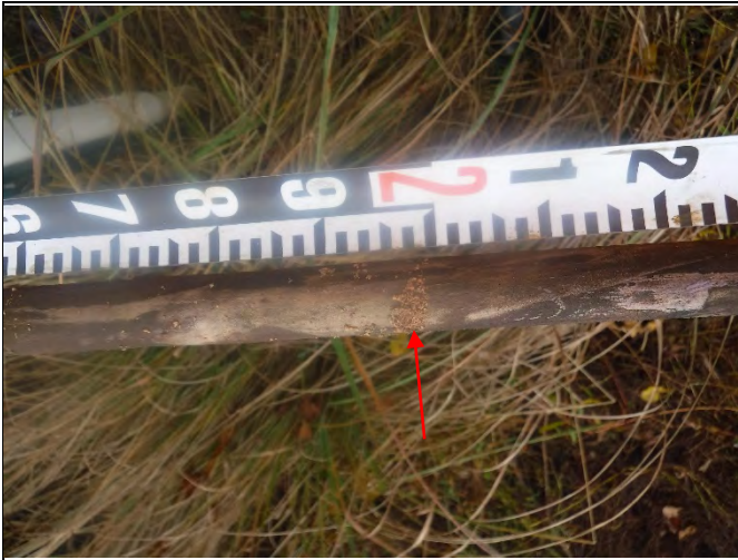
Crest Gauge Reach HC-R1: Close-up of gauge reading of 1.98' (photo from 11/13/20)
