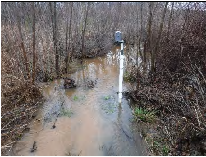
Flow Gauge in Reach UT4-R4b (photo 2/24/20)
