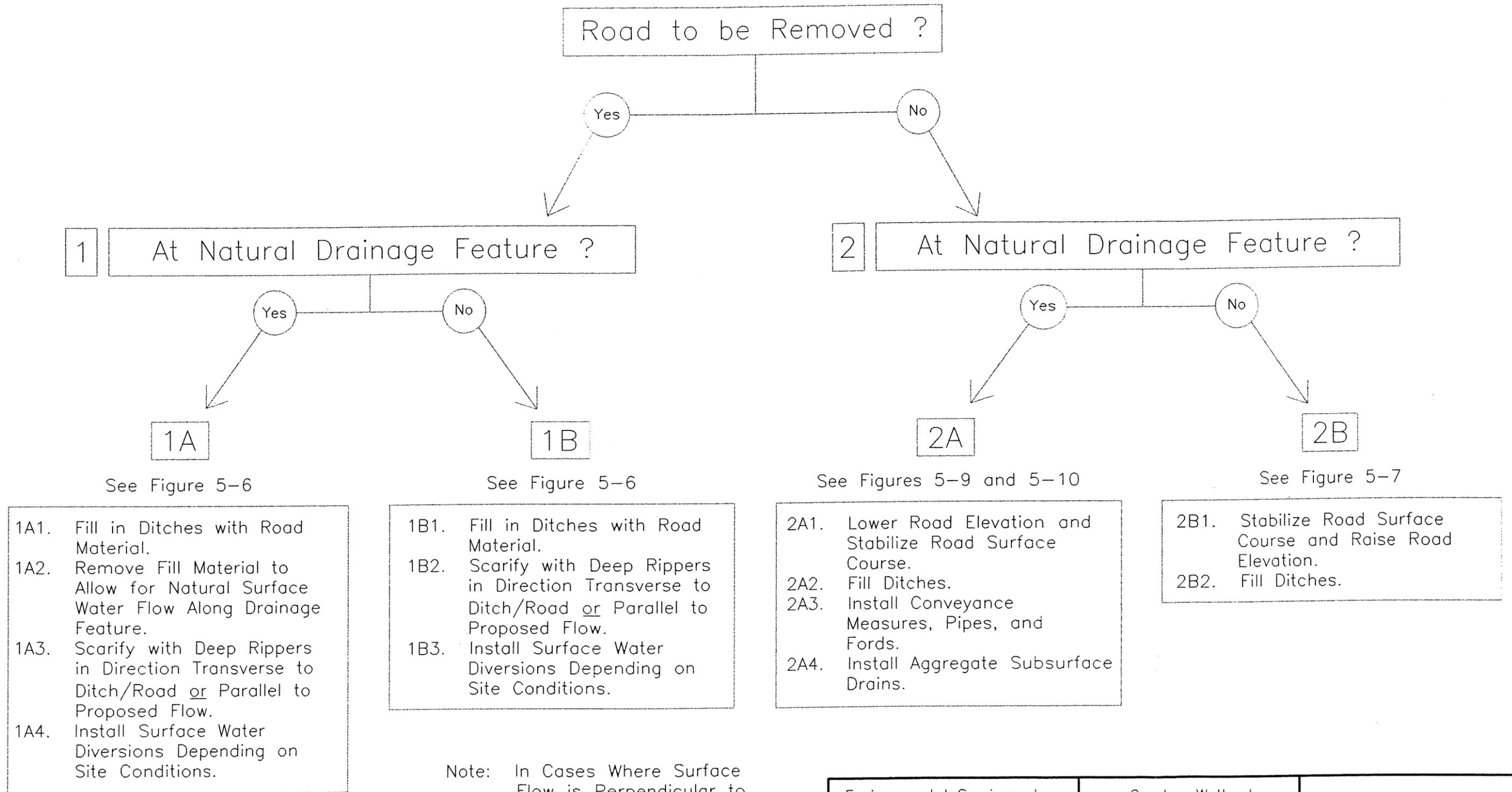
Note: In Cases Where Surface Flow is Perpendicular to Existing Channel Flow, Point Filling to be Used.
