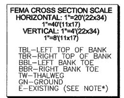
\*FEMA CROSS SECTION NOTE: **NOTE - SOME "EXISTING" ELEVATIONS** WERE TAKEN FROM THE EXISTING CONDITIONS SURVEY AND WERE NOT VERIFIED BY TURNER LAND SURVEYING.
