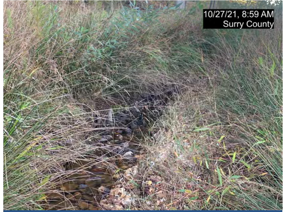
SPA8, R4, STA 20+75, Channel Bed Erosion (MY-02)
