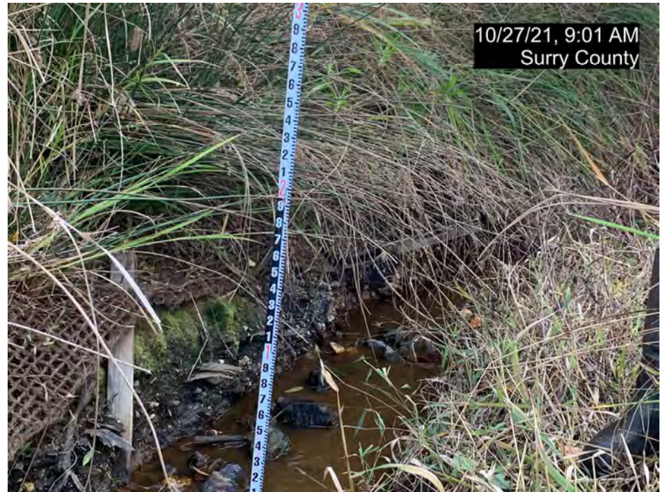
SPA8, R4, STA 20+75, Channel Bed Erosion (MY-02)
