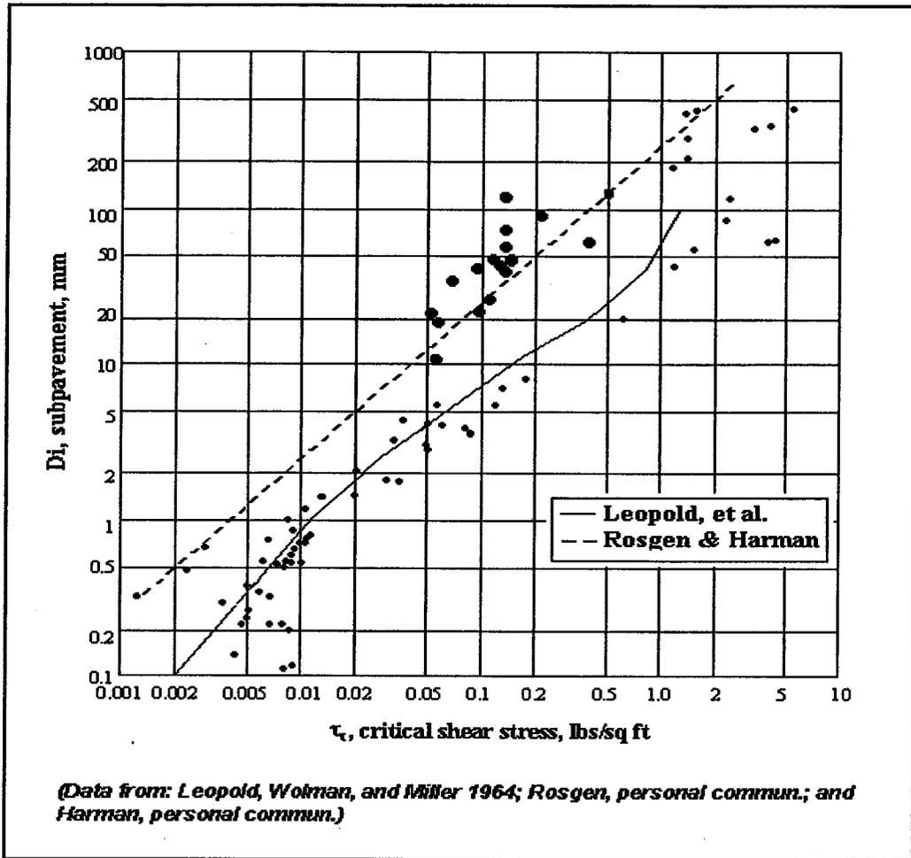
Figure 2.6.1 Modified Shield's Curve
