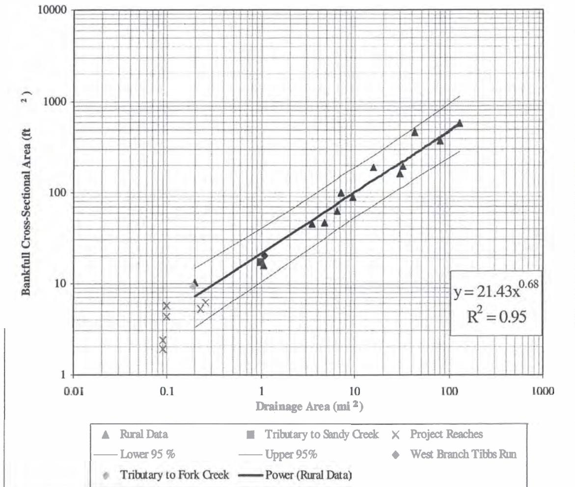
Figure 4.3 Rural Piedmont Regional Curve with Surveyed Bankfull Cross-Section Areas for the Tributary to Fork Creek, Tributary to Sandy Creek, West Branch Tibbs Run and Project Reaches. (Project data points were not used in determining the regression line.) (Harman et al., 1999)
