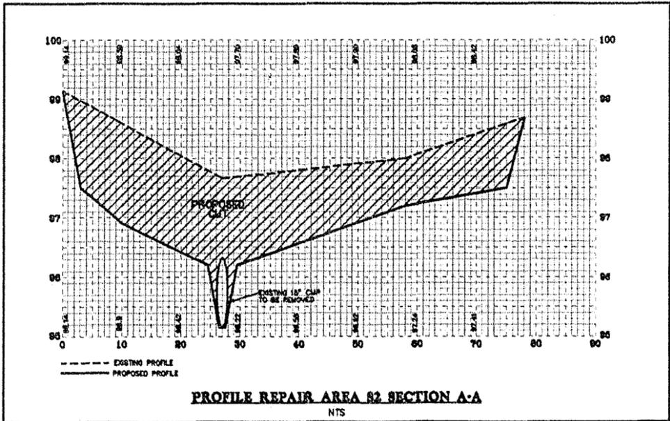
**PROFILE REPAIR AREA S2 SECTION A-A**
