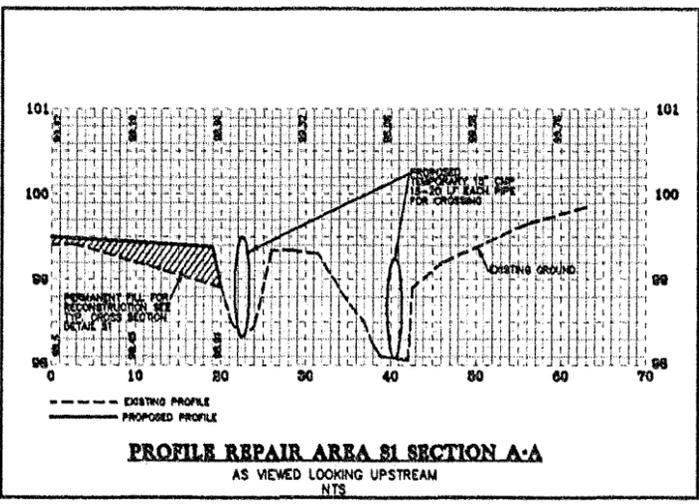
**PROFILE REPAIR AREA S1 SECTION A-A**
