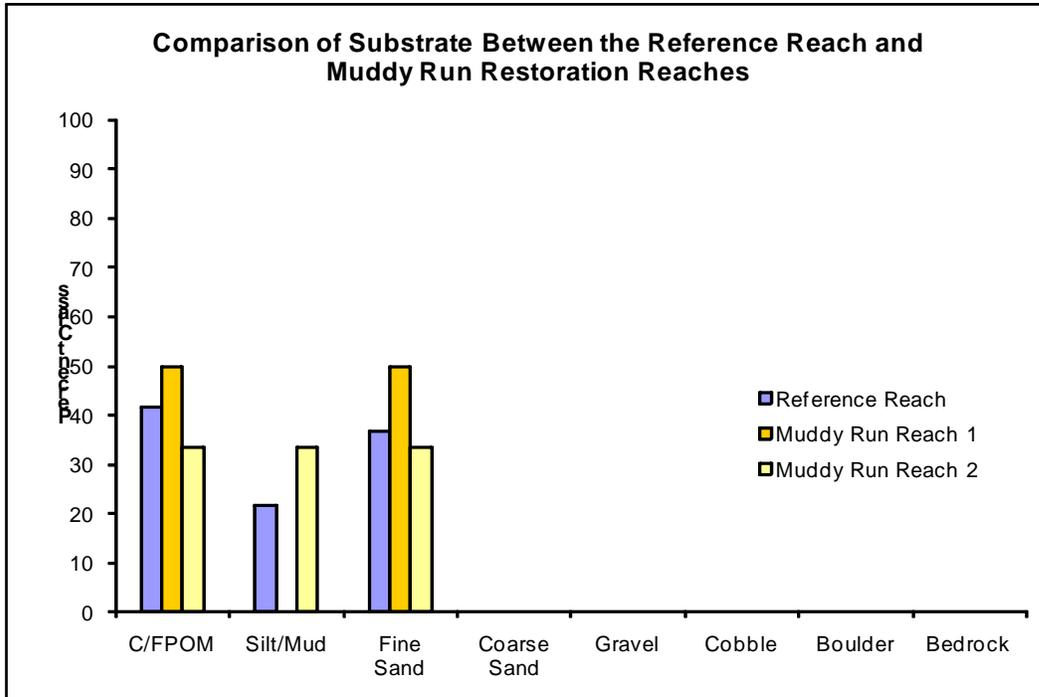
**Chart 3.** Comparison of substrate composition between the reference reach and the restoration reaches.
