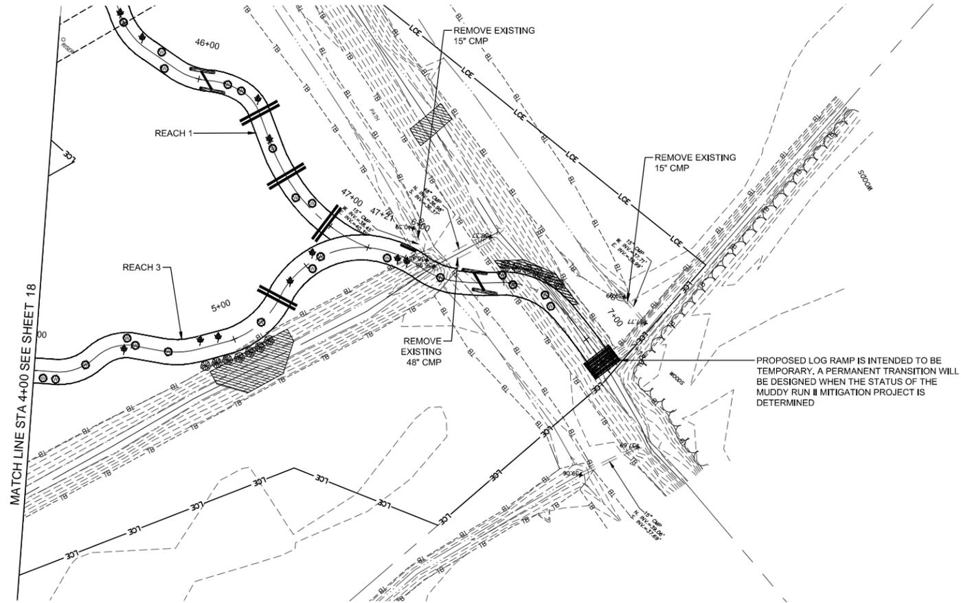
PROPOSED LOG RAMP IS INTENDED TO BE TEMPORARY. A PERMANENT TRANSITION WILL BE DESIGNED WHEN THE STATUS OF THE MUDDY RUN II MITIGATION PROJECT IS DETERMINED
