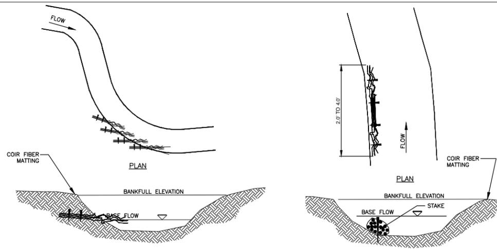
NOTE: WATTLES ARE TO BE INSTALLED 4' O.C. BY CUTTING AN APPROXIMATELY 4" WIDE TRENCH PERPENDICULAR TO THE STREAM BANK JUST ABOVE BASEFLOW ELEVATION. INSERT THE WATTLES, ANCHORING WITH STAKES, AND TIGHTLY BACKFILL WITH TOPSOIL. WATTLES SHALL CONSIST OF 5 TO 10 STEMS, 0.25" TO 0.5" IN DIAMETER. MINIMUM LENGTH IS 4.5 FEET. AT LEAST 3.0 FEET SHALL BE INSTALLED WITHIN THE BANK. WATTLES SHOULD BE INSTALLED AT AN ANGLE OF 20° TO 30° TO THE STREAM BANK AND SHOULD POINT DOWNSTREAM.
