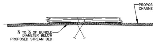
USE STICKS AND LOGS OF VARYING SIZES 1"-4" DIAMETER AND 1'-4" LONG. WOODY DEBRIS SHALL BE HELD IN PLACE USING TWINE AND WOODEN STAKES AND SHALL BE PLACED ACCORDING TO DESIGN PLANS AND AS DIRECTED BY ENGINEER.
