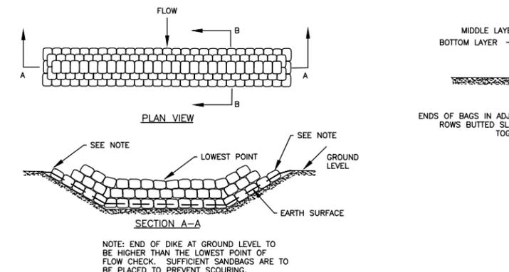
NOTE: END OF DIKE AT GROUND LEVEL TO BE HIGHER THAN THE LOWEST POINT OF FLOW CHECK. SUFFICIENT SANDBAGS ARE TO BE PLACED TO PREVENT SCOURING.
