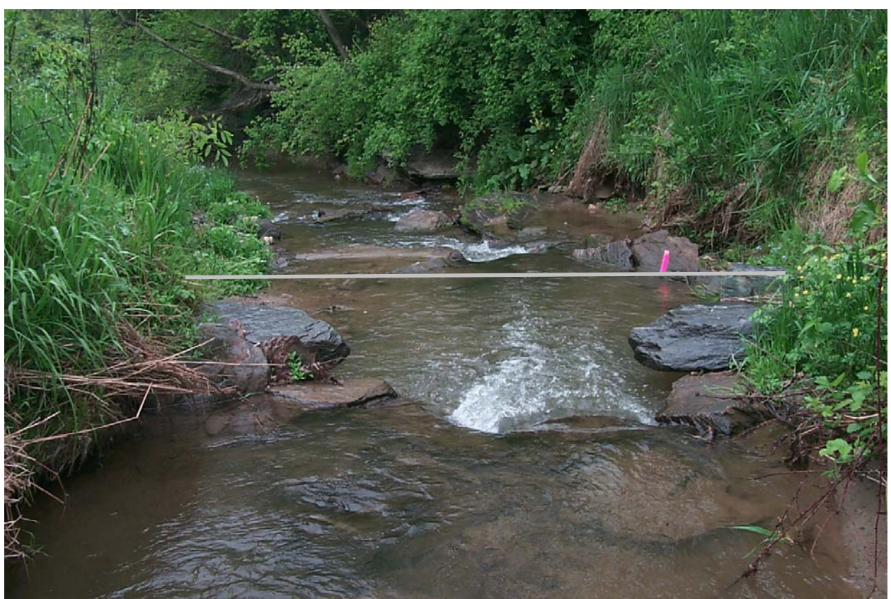
FIGURE 3.3.—Cross-section 7+13, step pool.
