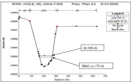
Figure 3.3 Cross-section and HEC-RAS Water Surface Elevations for Mountain Regional Curve Flow (75 cfs) and Higher Flow (100 cfs) at Cross-section of Sink Hole Reach 1
