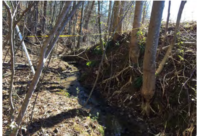
UT 2- cross section 2 in wooded area with high BHR and low ER.
