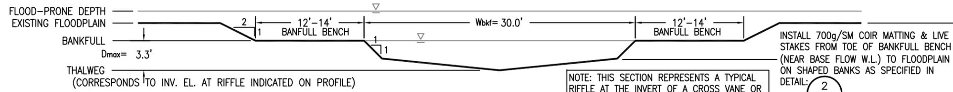
**SOUTH HOMINY CREEK (ALL REACHES): TYPICAL RIFFLE CROSS SECTION**
