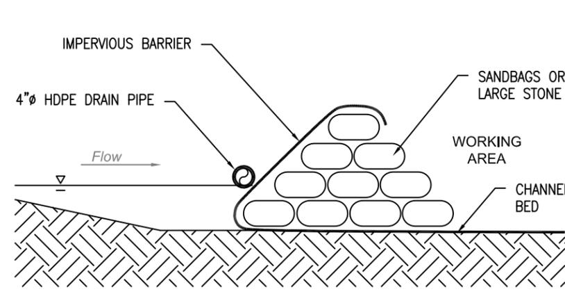
TEMPORARY IMPERVIOUS DIKE DETAIL
