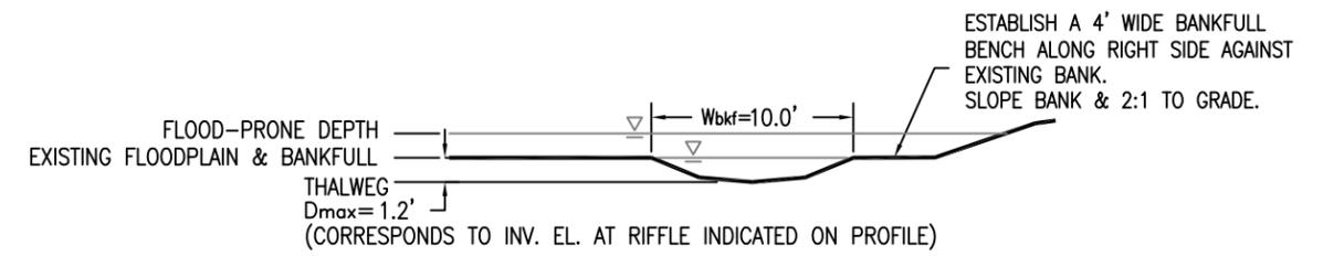
UT2-REACH 2: TYPICAL RIFFLE CROSS SECTION
