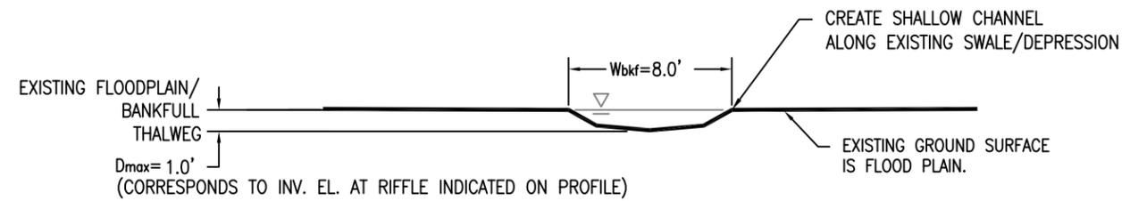
TYPICAL RIFFLE CROSS SECTION - UT1 REACH 2
