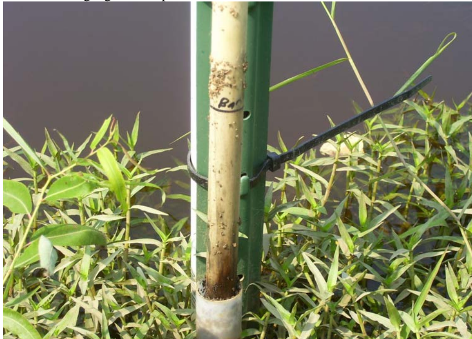
Photo 2. Crest gauge close up
