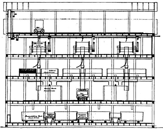
Fig. 28.-Chlorination plant at the Haile Gold Mine. Vertical Longitudinal Section.
