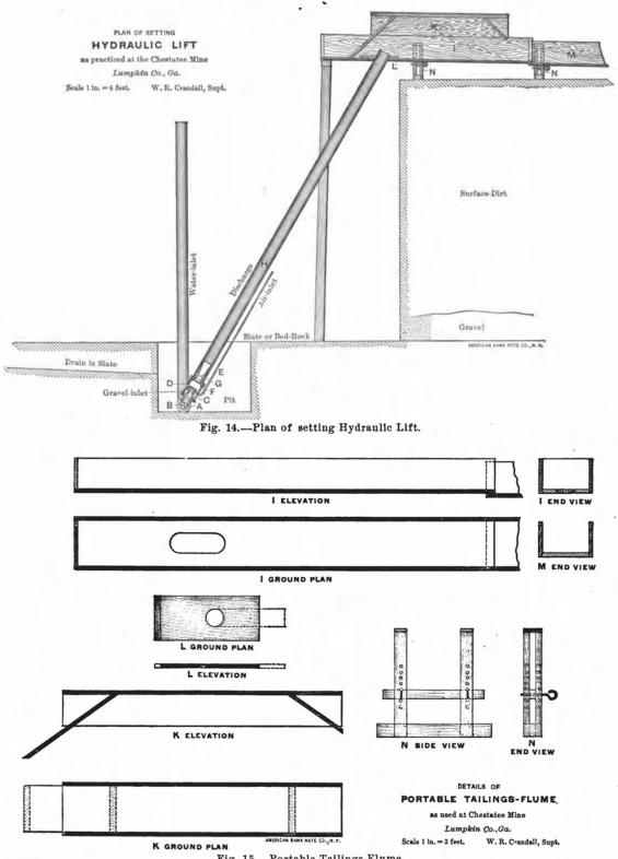
Fig. 15.—Portable Tailings-Flume.
