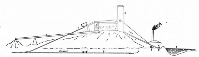
Fig. 6.—Sketch of method of working gravel at Crawford mine, Stanly county, N. C. (Not drawn to scale.) 1, reservoir; 2, pump; 3, hoisting engine; 4, stand-pipe; 5, washing-box; 6, grizzly; 7, sluices; 8, inclined plane; 9, track on bedrock.
