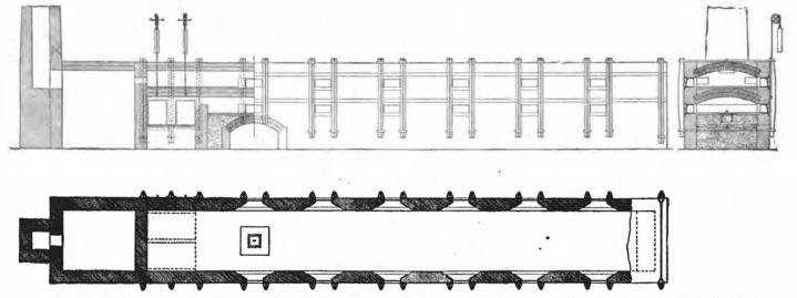
Fig. 27.—Double-Hearth Roasting Furnace; Chlorination Plant; Haile Gold Mine. Dimensions of hearth : 5 feet wide by 40 feet long. The upper figure represents a vertical, and the lower a horizontal section of the furnace.
