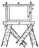
Fig. 10.—Flume, Mills Property, N. C. Scale,  $\frac{1}{2}$  lnch=1 foot. a, 1x3-inch board; b, 1-inch holes; c, 1x3-inch board; d, wedging; e, 1 $\frac{1}{2}$ -inch plank (sides and bottom); f, 2x4-inch sills and cap for bent.
