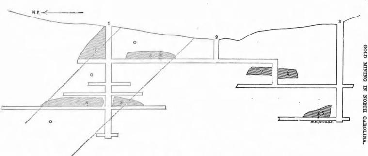
Fig. 18.--Vertical Section on the Strike of the Vein, Reimer Mine, N. C. Scale, 1 inch=80 feet. 1, shaft No. 1; 2, air-shaft; 3, shaft No. 2; O, dip of ore-shoots; S, stoped ground.
