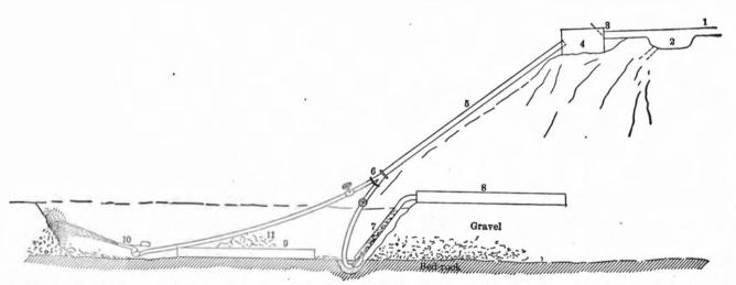
Fig. 9.—Sketch of proposed Hydraulic work on Mills Property, Burke County, N. C. (Not drawn to scale.) 1, ditch; 2, sand pit with drain; 3, screen at head of penstock; 4, penstock; 5, pipe (10 and 8-inch); 6, Y branching into two 7-inch pipes; 7, hydraulic elevator; 8, top sluice-boxes; 9, pit sluice-boxes; 10, giant; 11, bowlder and pebble heaps.
