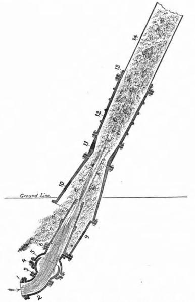
Fig. 11.-Hydraulic Gravel Elevator, J. C. Mills' land, Burke Co., N. C.
