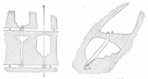
Vertical Section along Strike. Section on X-Y. Fig. 24.—Method of Stoping at the Cross Mine (Haile Mine). Scale, 1 inch=60 feet.
