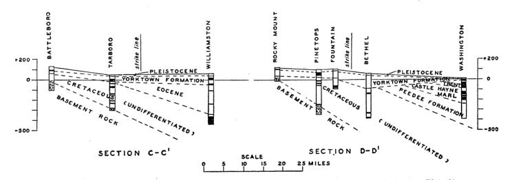
FIG. 3.—Cross sections along lines C-C' and D-D'. Water bearing horizons are shown in black. (see Plate 2)
