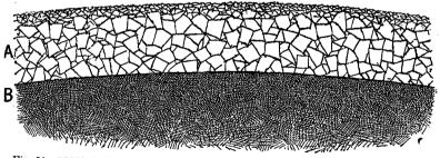
Fig. 23.—CROSS SECTION OF MACADAM ROADWAY (A) LAID ON COMPACT EARTH (B), MADE SOLID AND PERMANENT BY HEAVY ROLLING.
