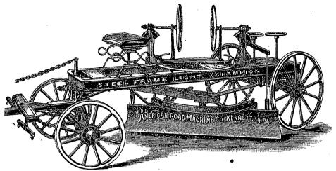
Fig. 34.-THE STEEL FRAME LIGHT CHAMPION REVERSIBLE ROAD MACHINE.
