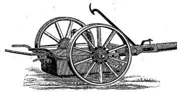
Fig. 33.-WHEEL SCRAPER IN POSITION FOR LOADING.
