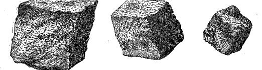
Fig. 20.—SHOWING ROUGH CUBE-SHAPED STONES OF PROPER SIZE AND FORM TO BE USED IN MACADAM AND TELFORD ROADS.—]From the Century Magazine].
