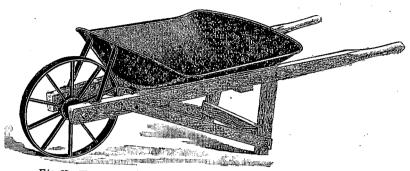
Fig. 27.-WHEELBARROW WITH IRON WHEEL AND PRESSED STEEL TRAY.
