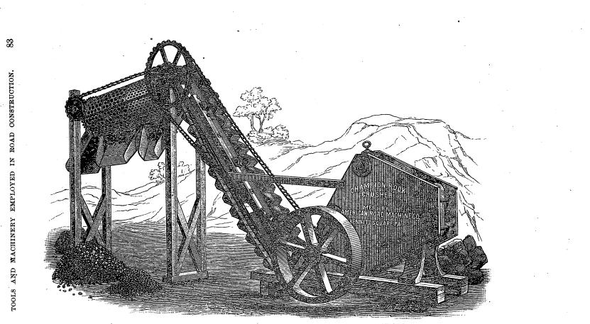
Fig. 41.-CHAMPION STEEL ROCK CRUSHER WITH ELEVATOR AND SCREEN ATTACHMENT.
