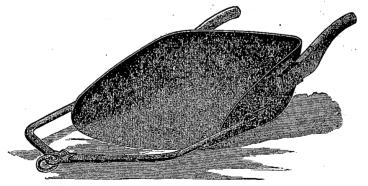
Fig. 30.-DRAG SCRAPER IN POSITION FOR LOADING.
