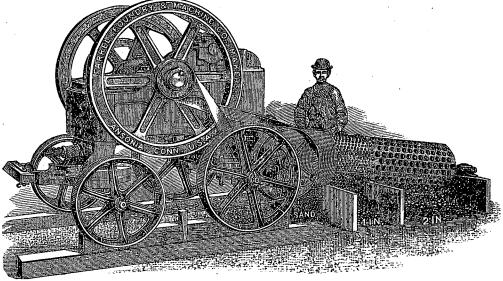
Fig. 38.—FARREL MARSDEN CRUSHER, MOUNTED ON WHEELS AND WITH SCREEN ATTACHMENT.
