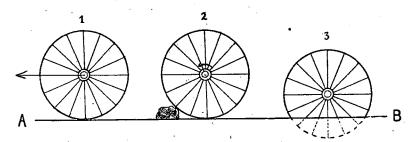
Fig. 7.—Illustrating the disadvantages of Bad Roads. No. 1 Represents a wheel on the smooth hard surface of a good road which offers very little resistance to the forward movement of the loaded vehicle. No. 2 is a wheel resting on the hard surface of a road covered with loose or permanent fragments of stone. No. 3 is a wheel partly sunk into the surface of a muddy road.
