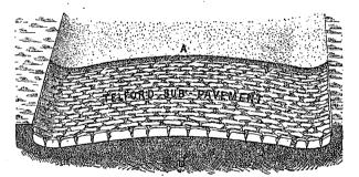
Fig. 15.—TOP VIEW AND CROSS-SECTION SHOWING METHOD OF CONSTRUCTING TELFORD ROADWAY. [From the Century Magazine.] B is the rolled earth foundation on which is laid the sub-pavementas shown in Fig. 14. At A have been laid the upper courses of broken stone rolled into compact form, similar to that shown in the broken-stone layer of Fig. 12.
