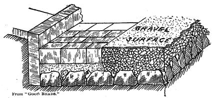
Fig. 22.—TELFORD ROAD SHOWING A FOUNDATION OF LARGER STONES WITH SMALLER STONES WEDGED BETWEEN THEIR TOPS; ON THE LEFT IS A PORTION OF CURBSTONE AND GUTTER AS USED IN CITIES, AND ON THE REGHT A PORTION OF THE BROKEN STONE COVERING OF THE ROADWAY WITH SURFACE GRAVEL. THE CURBSTONE AND GUTTER HERE SHOWN ARE TOO EXPLOSIVE FOR USE ON COUNTRY ROADS.
