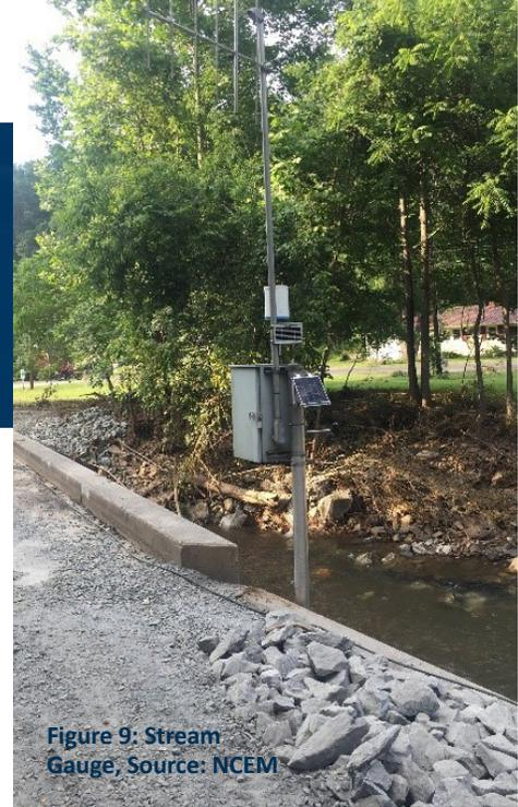
Figure 9: Stream Gauge, Source: NCEM
