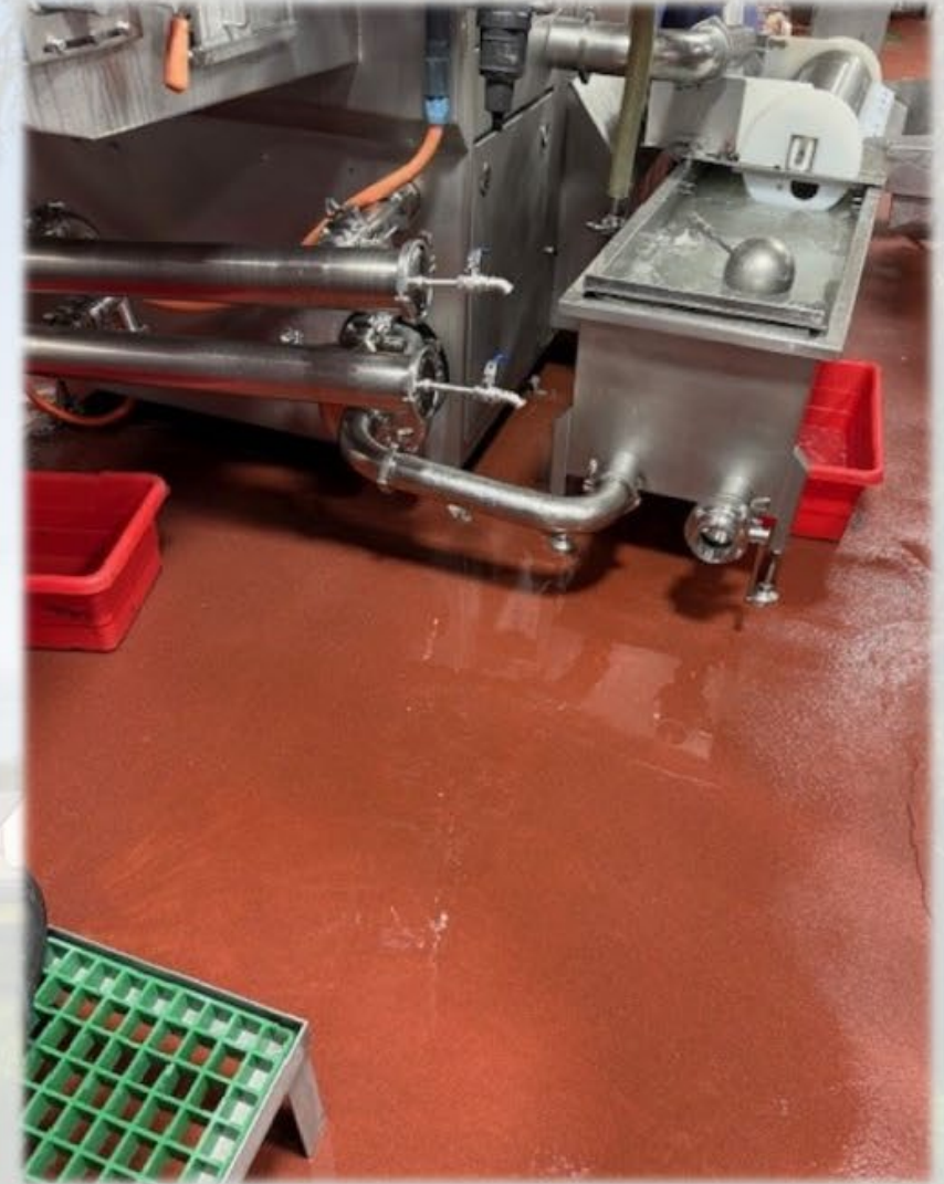
excessive brine on floor
