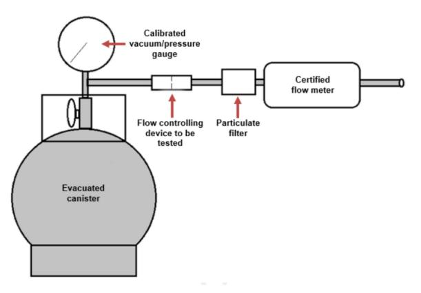
Figure 9-1: Flow controlling device characterization apparatus.
