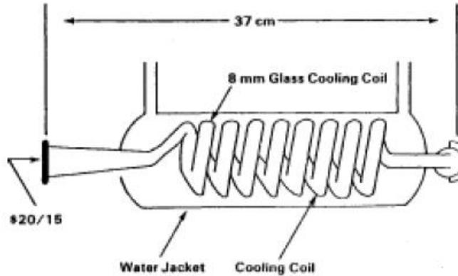
Figure 2 (Method 23 Type Condenser) Courtesy of the EPA
