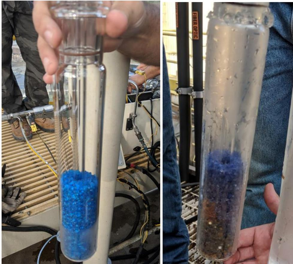
Picture 5 – Silica Gel Impingers [new (left) and nearly spent (right)]
