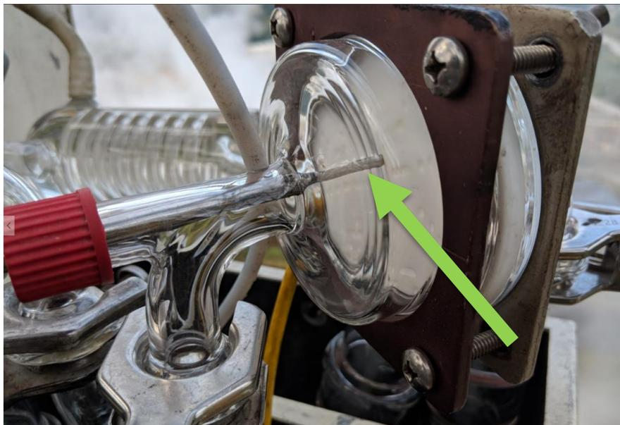
Picture 4 – CPM Thermocouple
