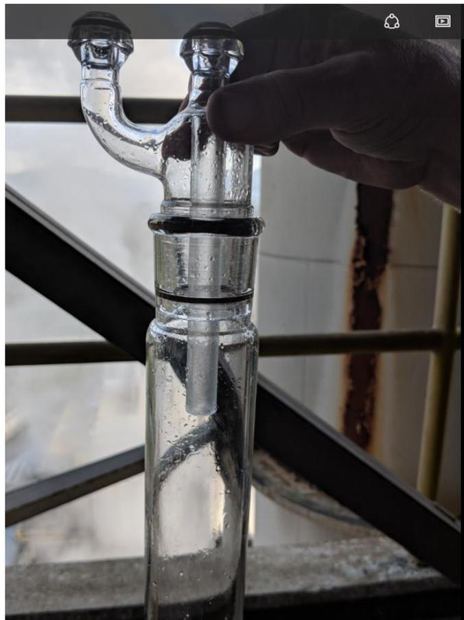
Picture 1 - Dropout Impinger
