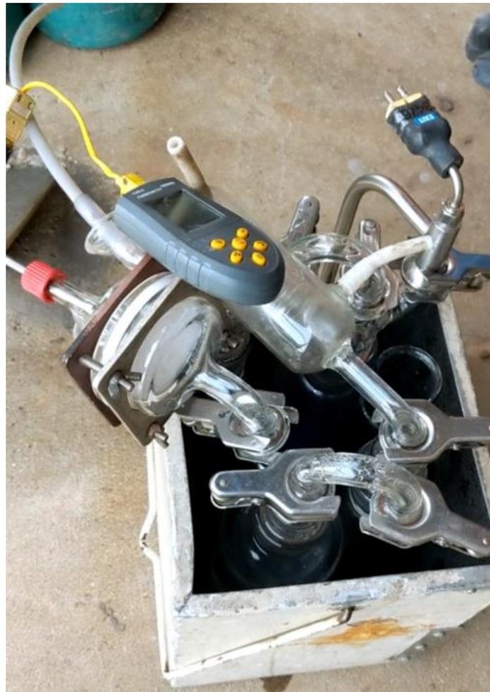
Picture 8 (Nitrogen Purge Setup – white line is N<sub>2</sub> gas coming from UHP nitrogen tank (green at top); temperature sensor pictured (device with yellow buttons))
