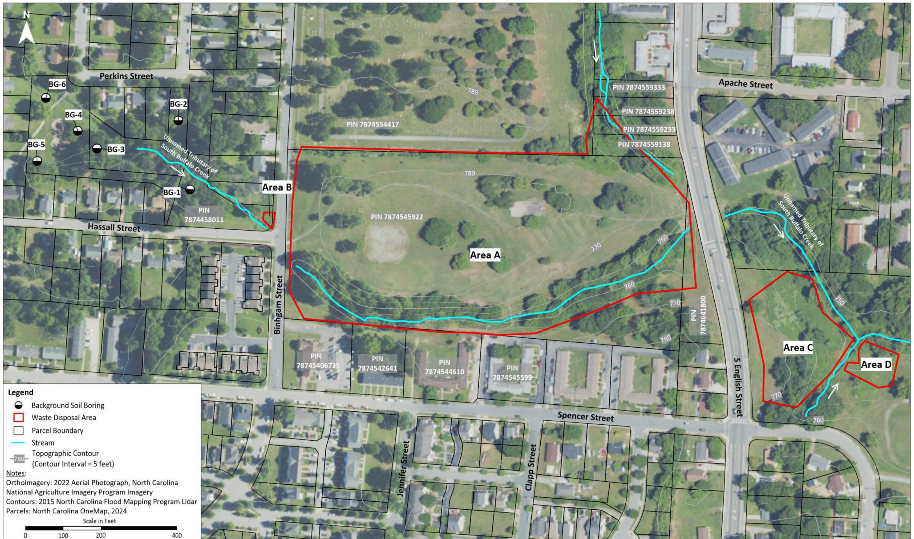
Figure 8-1 Background Soil Boring Locations
