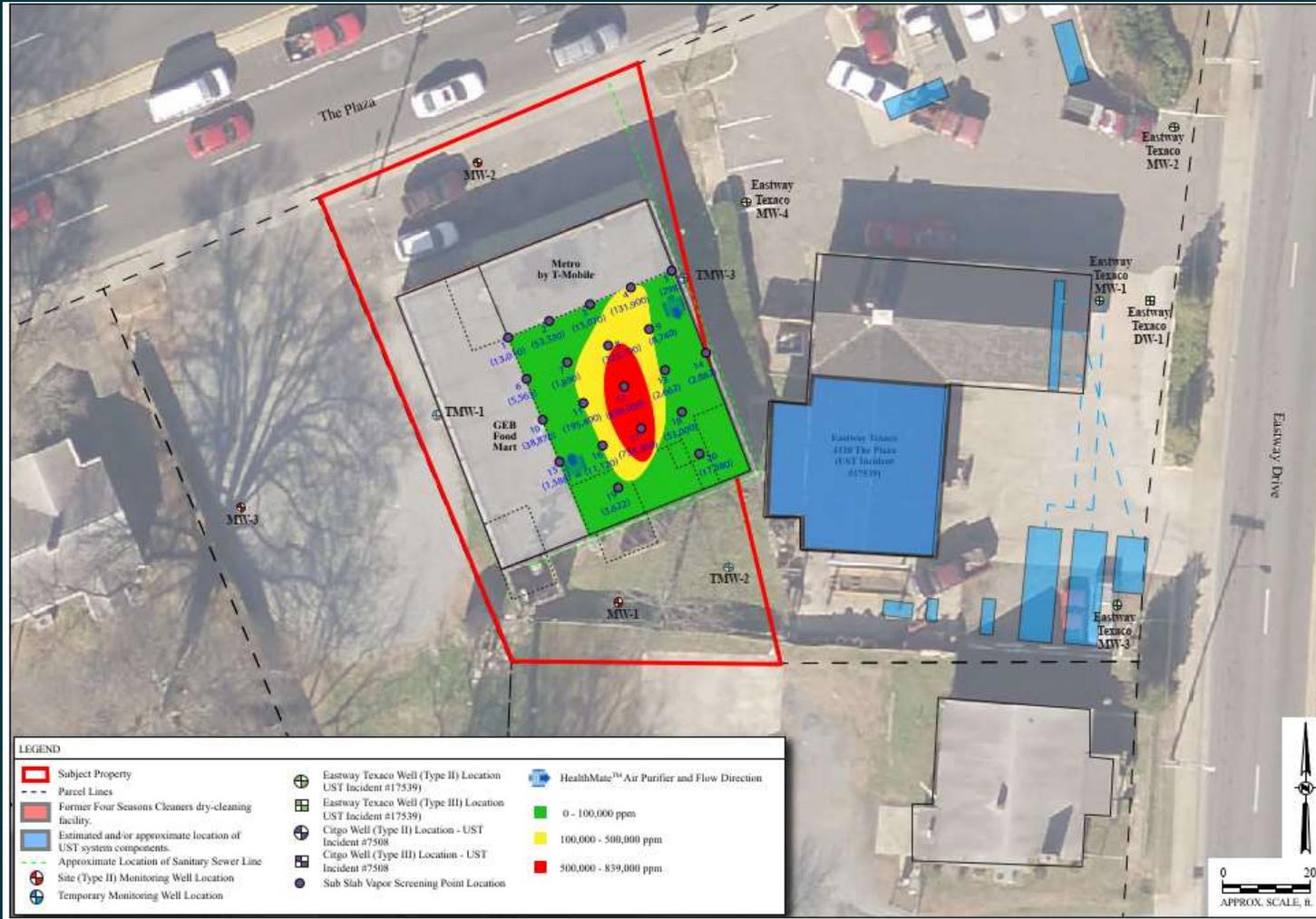
1. To further evaluate source areas at the site, we installed 20 temporary vapor monitoring points in a gridded array and screened total vapor concentrations beneath the slab
