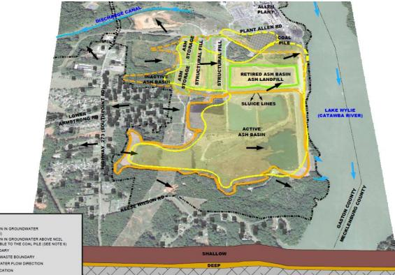
Groundwater flow is determined by monitoring well data (elevations and levels of constituents.)
