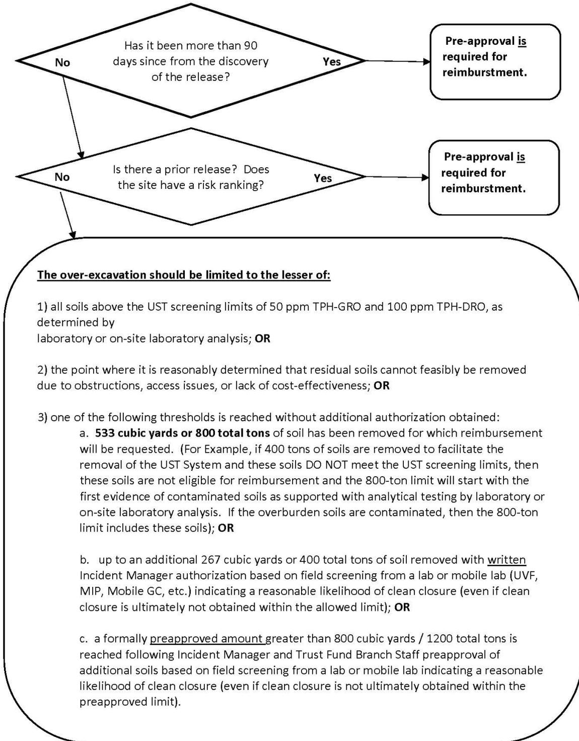
**Figure 9 -Soil Excavation for Initial Abatement of a NEW ISOLATED Release at a Site with a Prior Release, Risk Ranking AND USTs are Being Permanently Closed (or do not Impede Soil Excavation) - Pre-approval Required**
