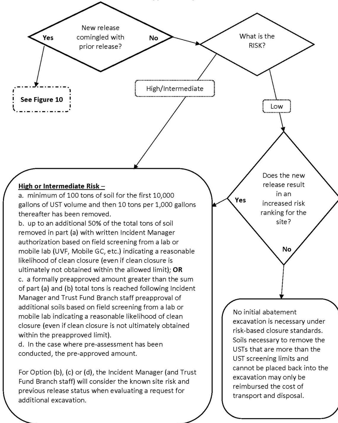
**Figure 10 - Soil Excavation for Initial Abatement of a NEW COMINGLED Release at a Site with a Prior Release AND Risk Ranking AND USTs are Being Permanently Closed (or do not impede soil excavation) - Pre-approval Required**
