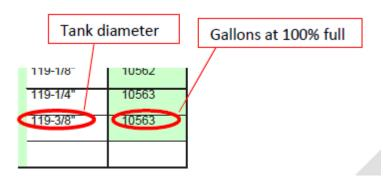
Next look at the tank chart for the gallons that corresponds with the height the ball float vent valve is set at.
