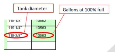
Next look at the tank chart for the gallons that corresponds with the height the ball float vent valve is set at.
