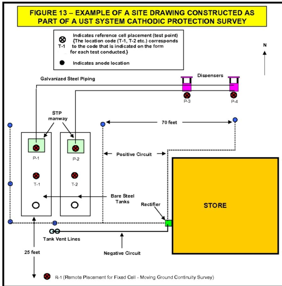
While it is understood that the CP contractor will not always know where all of the pertinent components of the cathodic protection system may be buried, all that is known must be indicated. It is very important to show where the anodes are located on the site drawing. If it is not known where the anodes are buried, voltage gradients in the soil may help you determine the approximate location as described in the raised earth discussion of Section 6.3.
