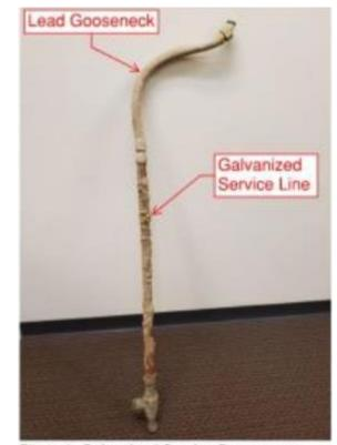
Photo 1: Galvanized Service Downstream of Lead Gooseneck (CFPUA Typical)
