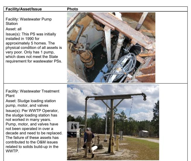
Figure 4-3. Asset Condition Assessment Example 2 (Submersible Pump Station and WWTP Sludge Loading Station)
