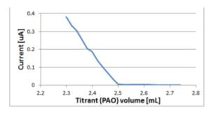
The results are calculated with the sample volume used, the concentration of the PAO, and the volume of the PAO needed to reach the end point (which is where the graph goes from sloped to flat and the µA reading no longer changes). [Hach® Document TE728,2 Version 4.0, published 4/10/2018]
