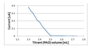
The results are calculated with the sample volume used, the concentration of the PAO, and the volume of the PAO needed to reach the end point (which is where the graph goes from sloped to flat and the  $\mu$ A reading no longer changes). [Hach® Document TE728,2 Version 4.0, published 4/10/2018]
