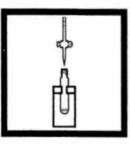
7. Add a stir bar and titrate with the Ferrous Ammonium Sulfate Standard Solution selected in Step 4 until the color changes from greenish-blue to orange-brown. Record the number of mL required. This is value C in the following equation.
