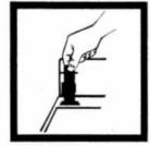
4. Place the COD Vial Adapter into the cell holder with the marker to the right.
