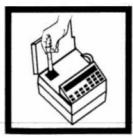
9. Piace the sample vial in the adapter with the Hach logo facing the front of the instrument. Place the cover on the adapter.
