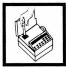
9. Place the sample vial into the adapter with the Hach logo facing the front of the instrument. Place the cover on the adapter.
