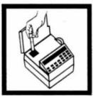
6. Place the blank into the adapter with the Hach logo facing the front of the instrument. Place the cover on the adapter.
