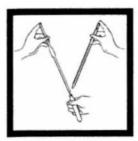
5. Pipet 2.00 mL of Potassium Dichromate Standard Solution into an empty vial. When using the Low Range COD Digestion Reagent Vials, use a 0.025 N solution. When using High Range or High Range Plus COD Digestion Reagent Vials, use a 0.25 N solution.
