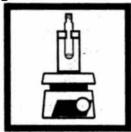
3. Place the vial on the titration stand. Turn on the magnetic stirrer.
