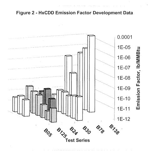
While the TCDD toxicity potency is ten times that of HxCDD, the risk assessment results for wood-fired boilers are driven by HxCDD. From Table 1 it can be shown that the emission factor for HxCDD is 3400 times higher than TCDD. Table 2 presents the emission factor, potency factor, and the multiplication product of these two factors to illustrates why HxCDD drives the risk assessment so much more than TCDD.
