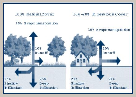
The relationship between in pervious cover and surface runoff: Hardened surfaces in a watershed result in increased storm water runoff because the water is notable to soak into the ground. The runoffpicks up pollutants as itm oves over in pervious surfaces making itm ore likely that our waterways will receive harm fulpollutants.
