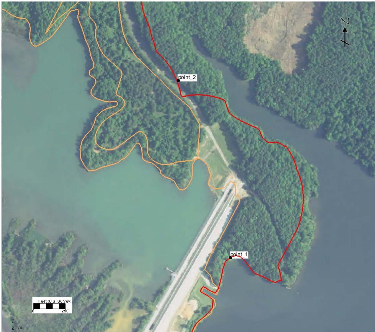
Figure 6-7. Locations for boron time-series plots (point 1 and point 2). The red line is the current compliance boundary and orange lines are waste boundaries and landfill boundaries.
