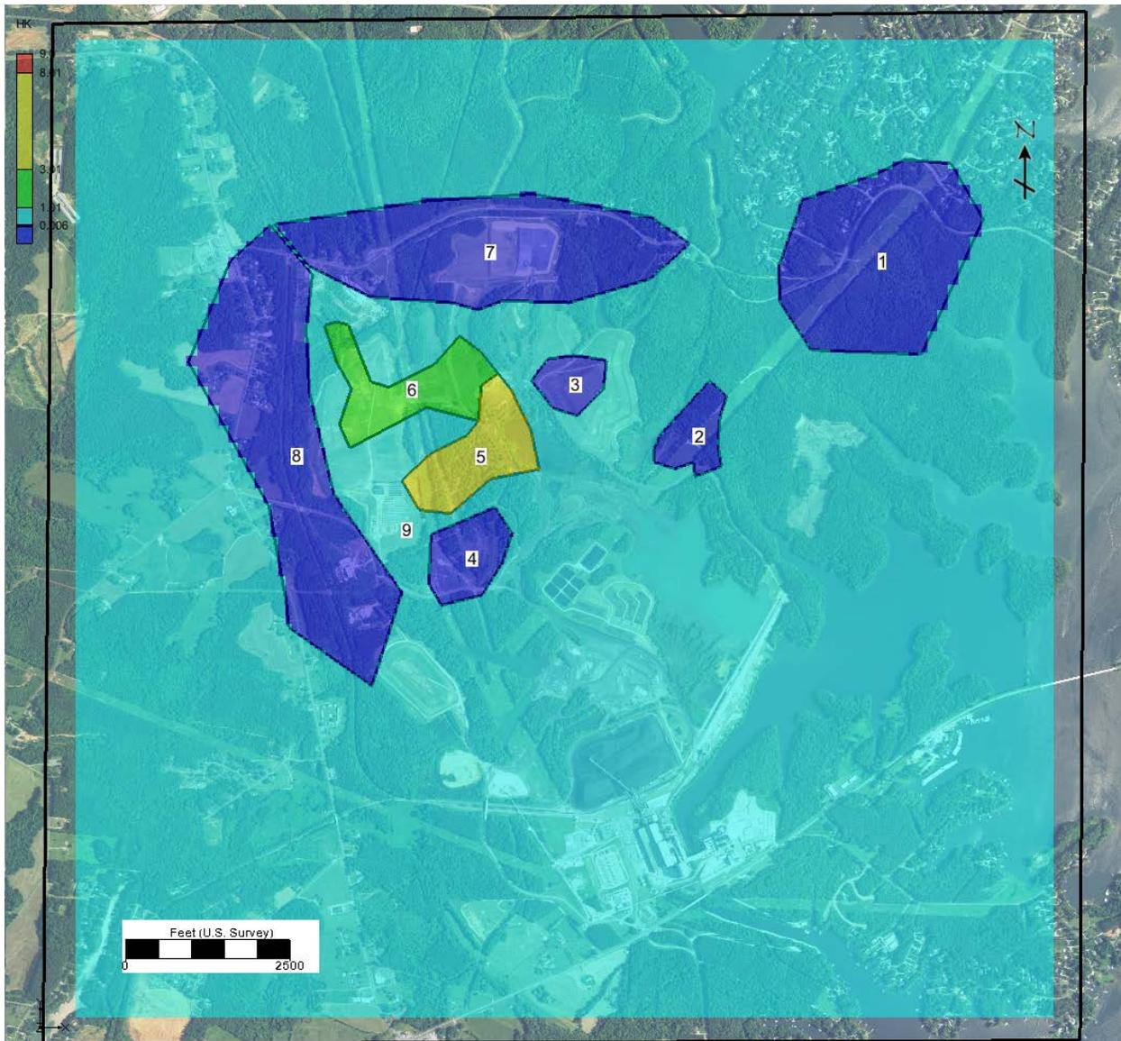
Figure 5-4. Zones used to define horizontal hydraulic conductivity and horizontal to vertical anisotropy in the upper bedrock, model layer 9.
