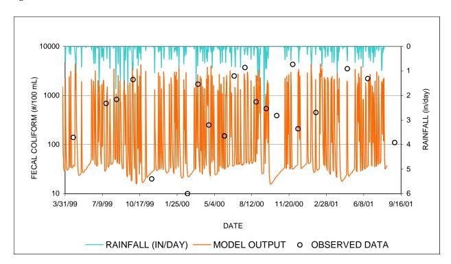
Figure 5. Simulated versus observed fecal coliform concentrations from 3/1999 to 8/2001
