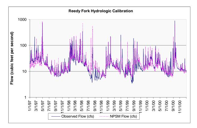
Figure 3. Simulated and observed flows recorded at USGS 02093800 Reedy Fork, 1997-2001.
