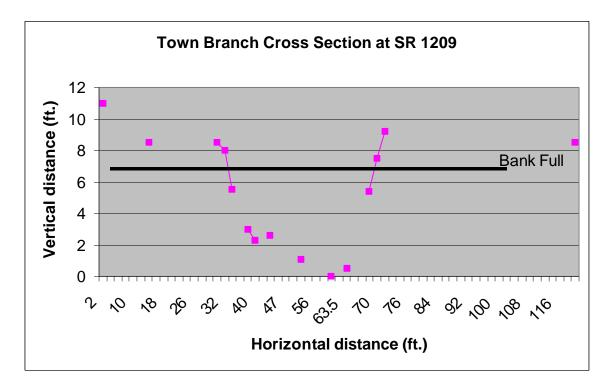
This cross section was used to develop the model F-table (table that describes relationship between streamflow depth and streamflow volume).
