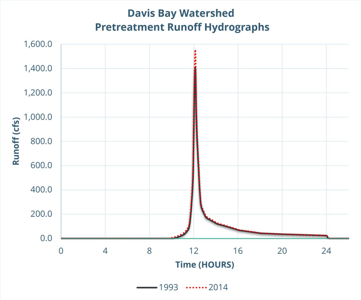
Figure 3-1. Pre-treatment runoff hydrograph of Davis Bay Watershed comparing 1993 rates to 2014.
