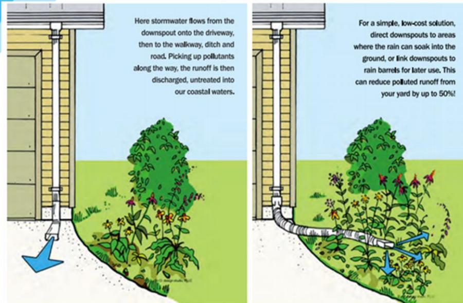
**Downspout disconnectors:** If a downspout from a gutter empty into a driveway, sidewalk, or parking lot, simply **re-directing the downspout** to an area that can filter the water naturally will reduce polluted runoff. A flexible downspout extension can be purchased at a local home improvement store for **less than \$10**, and used to direct water to vegetated areas. Directing rainwater to a lawn or garden that normally needs watering could result in **savings on your water bill**.
