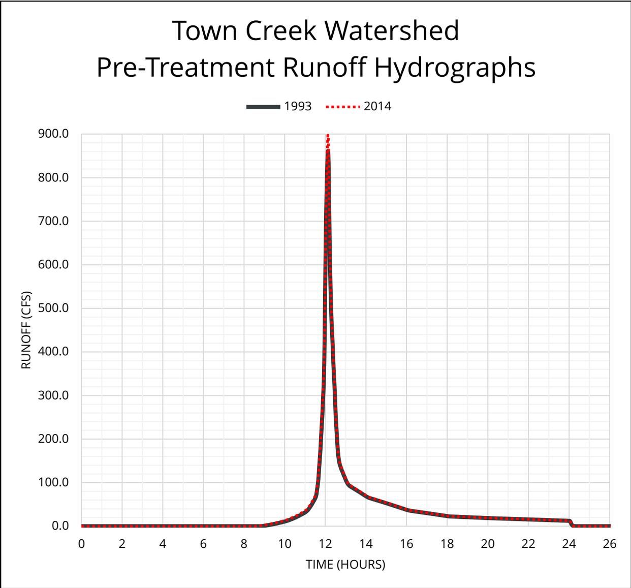
Figure 3-3. Pre-treatment runoff hydrograph of Town Creek Watershed comparing 1993 rates to 2014.
