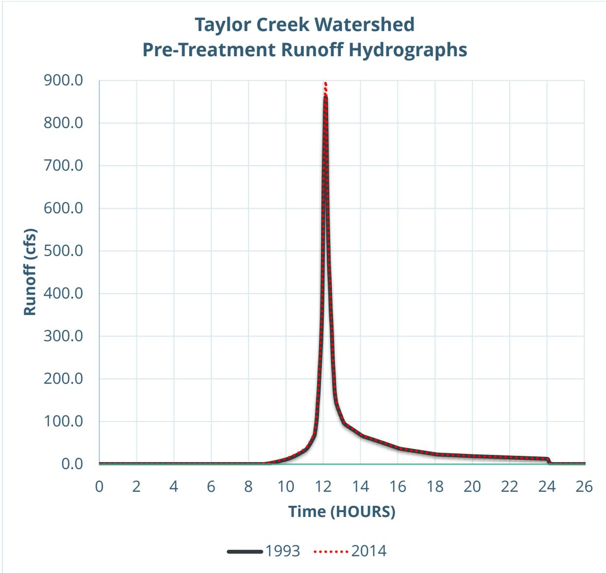
Figure 3-2. Pre-treatment runoff hydrograph of Taylor Creek Watershed comparing 1993 rates to 2014.
