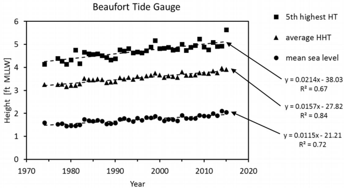
Figure D-8. The historical trend in tidal heights at Beaufort, NC. Mean sea level is the average of all hourly data for that year.
