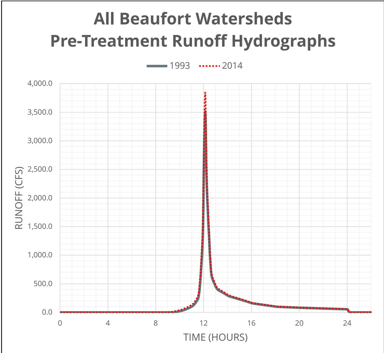
Figure 3-1. Pre-treatment runoff hydrograph of Beaufort Watershed comparing 1993 to 2014.
