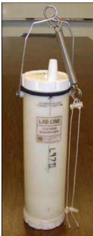
Figure 2. Labline sampler for photic zone (vertical spatial) composites.
