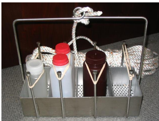
Figure 4. Cage sampler used in the DWR Ambient Monitoring Program
