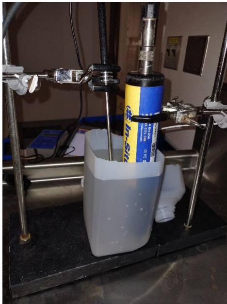
Figure 36. In-Situ Thermistor Check Ice Bath Procedure
