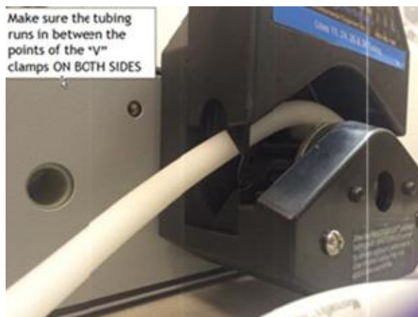
Figure 23. Loading the Tubing in the Peristaltic Pump.
