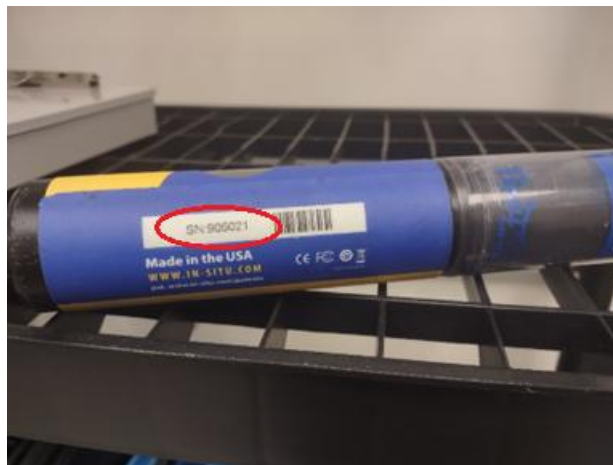
Figure 18. The In-Situ Field Meter Multiparameter Probe Serial Number Location.
