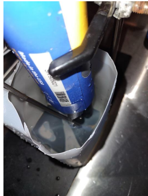
Figure 36. In-Situ Thermistor Check Ice Bath Procedure
