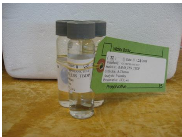
Figure 9. Labeling Multiple Vials as a Set with Rubber Band, Tag, and Label
