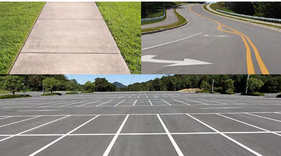
Figure 2: Examples of impermeable surface: (left to right): Concrete, Street/Roads, & Parking Lots.
