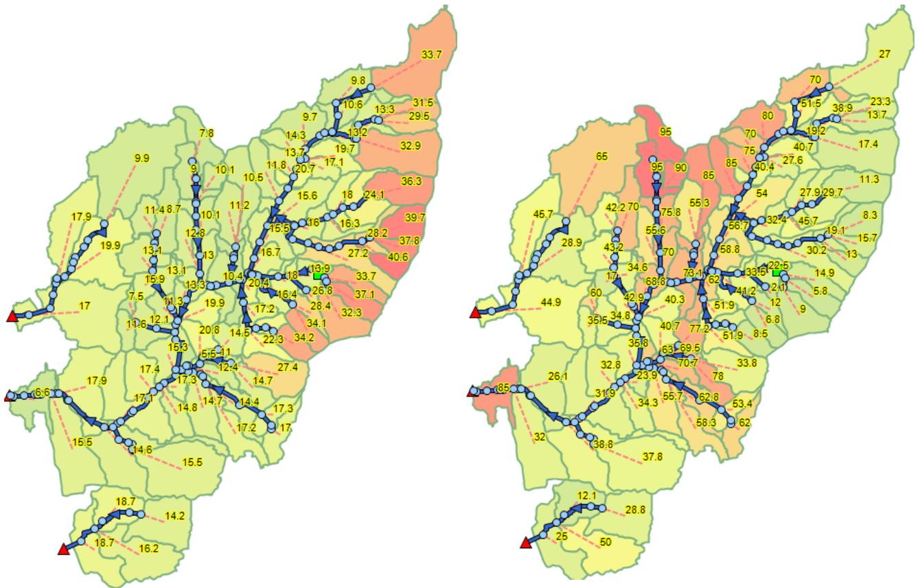
Figure 7 CAW catchment slope (%) (left) and impervious percentage (right). Note that the blue lines and circles on this map represents the larger pipes of the City's stormwater system and the watershed's streams.
