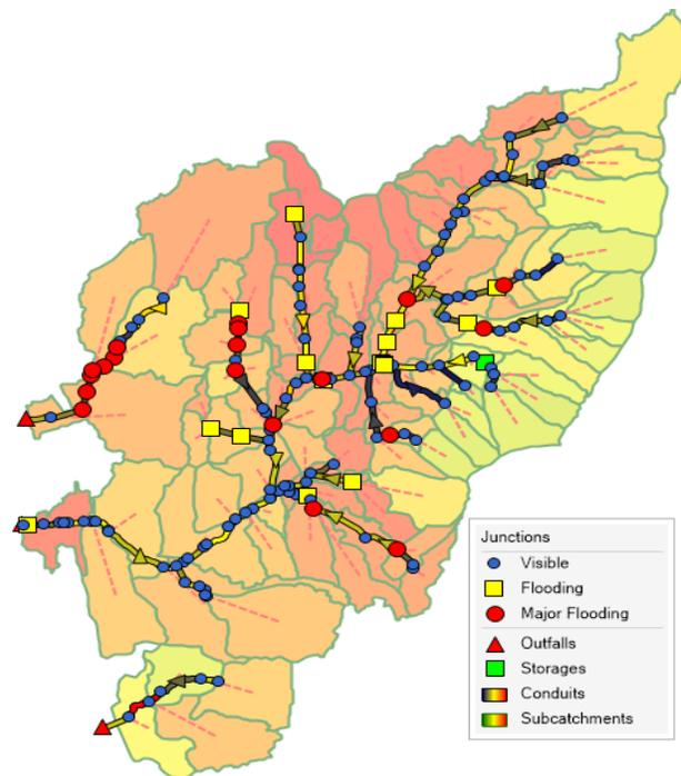
Figure 18 Flooding in the watershed for the 25-year
