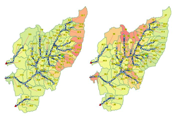
Figure 7 CAW catchment slope (%) (left) and impervious percentage (right). Note that the blue lines and circles on this map represents the larger pipes of the City's stormwater system and the watershed's streams.
