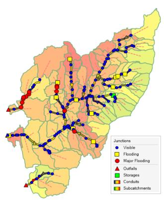
Figure 17 Flooding in the watershed for the 10-year
