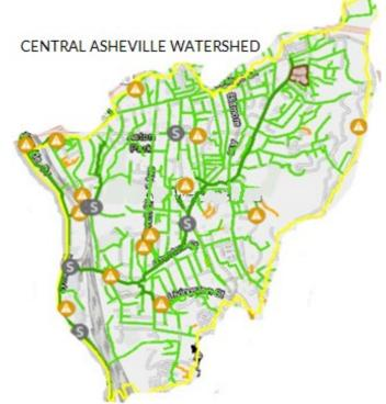
Figure 13 MSD Sanitary lines in the CAW and reports of SSO (denoted by an S) and Odor problems (denoted with triangles) in the past three years.
