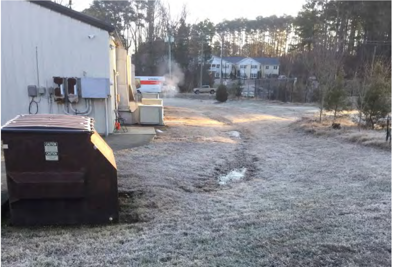
Figure 4-4. Potential new SCM site in which a wet swale was recommended (SCM Site NHC0014 located along Garrett Rd. within the Lower New Hope Creek watershed). A proposed 650-foot-long treatment swale would collect runoff from an adjacent commercial parking lot and roof.
